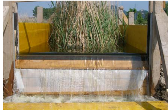
Figure 7: The downstream adjustable weir.
