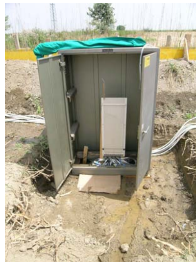
Figure 8: The differential piezometer system for water depth measurement.
